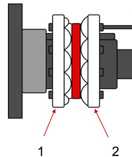
5. We remove the roller from the shaft and we rotate it so that the front part is positioned behind and then we put it in again.
