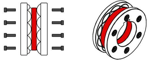
3. Next we place the outer spacer 8 on the upper machine shaft.
