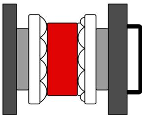
**Rollers assembling for 50mm o 2" handrail**
