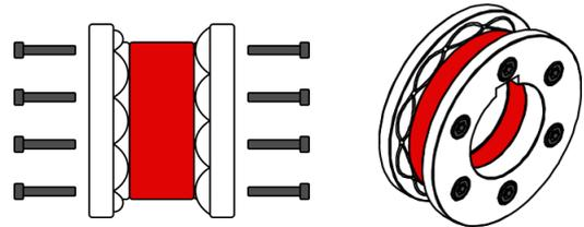
3. Next we place the outer spacer 10 on the upper machine shaft.
