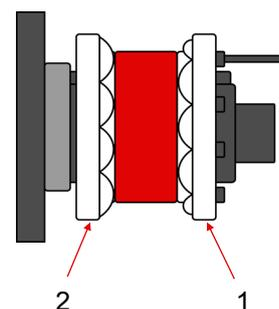
7. We remove the roller from the shaft and we rotate it so that the front part is positioned behind and then we put it in again.
