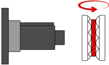
8. Next we place the outer spacer 8 on the upper machine shaft.
