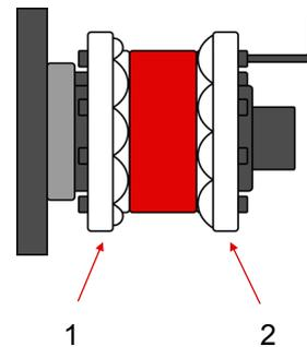
5. We remove the roller from the shaft and we rotate it so that the front part is positioned behind and then we put it in again.
