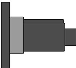
4. Place the pre-mounted roller on the upper axis and tighten the bolts with the Allen key.
