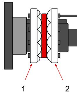
5. We remove the roller from the shaft and we rotate it so that the front part is positioned behind and then we put it in again.
