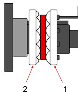
7. We remove the roller from the shaft and we rotate it so that the front part is positioned behind and then we put it in again.
