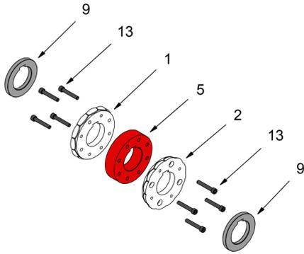
2. We do a pre-assembly, without tightening the bolts, paying special attention in aligning the slots for the pin.
