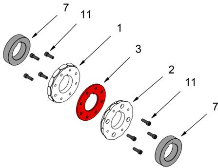
2. We do a pre-assembly, without tightening the bolts, paying special attention in aligning the slots for the pin.
