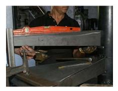
7. We level the step so that it is completely parallel to the ground.
