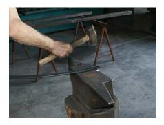
14. The handrail is twisted with a mallet to give it the perfect curvature.
