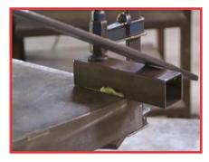
The secret to bending the railing both in the tube and in the handrail is to leave the rollers or wheels of the rollers free. That is to say if we introduce the tube by the end of the right, the roller of the left part of the machine must be without any type of subjection so that the rail of tube or handrail can take the suitable inclination. The tube of the rail comes out bent in a spiral form when being forced by the lateral supports.
