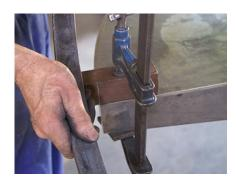
13. Check that the railing fits with the marks of the tooling.
