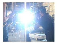
10. Proceed to permanently weld the step to the central tube. In this way we fix all the steps up to the proposed height.
