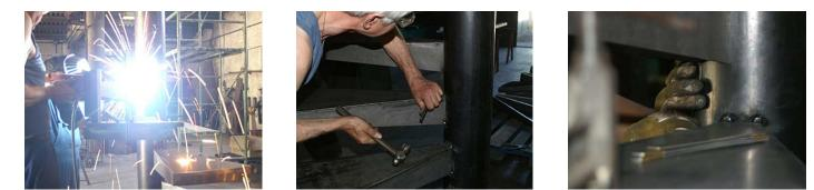
8. The step is fixed to the central tube with four welding points.
