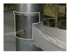
5. We use a round square made to measure that we fix to the tube, where the step will rest while we fix it.
