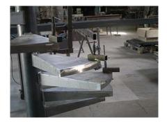
11. Next we have to manufacture the handrail of the spiral staircase. A tooling to which we mark the distance and the thickness of the handrail is fixed to the steps. These pieces allow to adjust the railing in an exact way.
