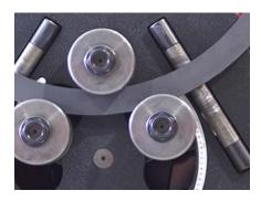
12. The MC400 Tube and Profile Roller is in charge of curving the handrail, giving it the exact shape without damaging it.
