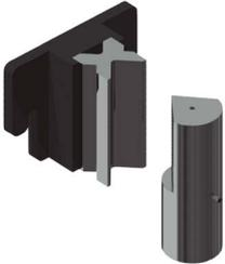
> Folding or bending die up to 161mm with 4 openings (16, 22, 35, 50mm) and a punch of 80°. This multi-V die allows 1mm up to 8mm sheet to be folded. The 70mm outer diameter punch allows to make completely closed shapes to a minimum of 75mm inner wing.
