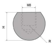
Radius elements to fold. Made of C45, a high quality, medium grade steel, with constant mechanical properties and good external chrome resistance.
