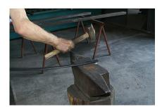
4. The handrail is twisted with a mallet to give it the perfect curvature.
