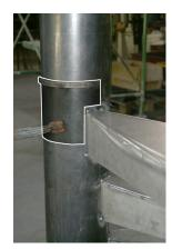
5. We use a round square made to measure that we fix to the tube, where the step will rest while we fix it.
