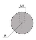
Radius elements to fold. Made of C45, a high quality, medium grade steel, with constant mechanical properties and good external chrome resistance.
