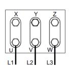
Triangle figure For voltage 230V
