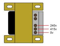
Figure 8. Change transformer primary connection
