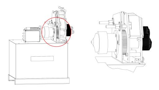
Figure 3. Mechanism protection guards
