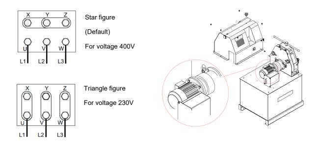
Figure 7. Change of engine connections
