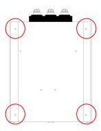
Figure 5. Anchor points of the machine
