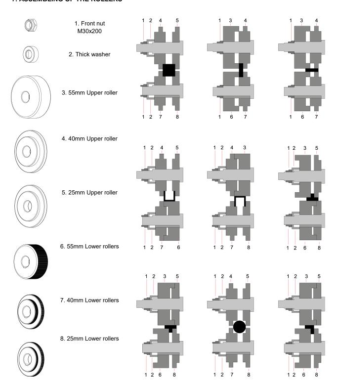
Figure 12. Nomenclature of the rollers and assembly
